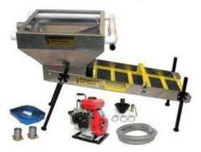
A highbanker is basically a sluice box with mobility and added height. It is mounted on a 4-legged stand that gives the sluice box the correct slope. Instead of being put right in the creek like a sluice, an engine with a water pump and some hoses transports the water up from the stream into the highbanker. Highbankers are also called <u>power sluices</u>. It is a self-contained unit with many uses— prospecting, sampling, and concentrate clean up.
